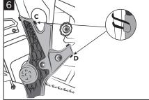
Fasten the left X-Grip using one big O-ring (C) and one little O-ring (D).
