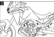
Remove the left original cover by unscrewing the screw (F).
