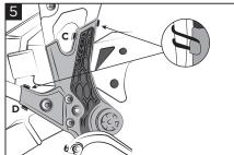
Fasten the right X-Grip using one big O-ring (C) and one little O-ring (D).
