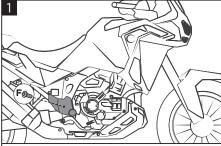
Remove the right original cover by unscrewing the screw (F).
